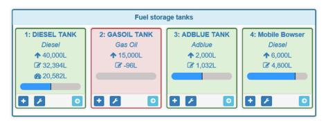
If a gauge is fitted (as on tank 1 here) there is an additional line showing the volume in the tank according to the tank gauge. A tank with a gauge is highlighted by the graphical contents display being lower than on those without.
