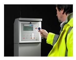
The Fuel Island Controller is the user interface for the pumps on site. Before fuelling the user must ID the vehicle to be fuelled (eg using a tag or card) and then may be prompted for other information such as mileage or registration number. The fuel island is configured to match the site it is installed on so that it can make decisions on what pumps to offer, or what ID methods to accept. This set up is only required once, when the system is installed.
